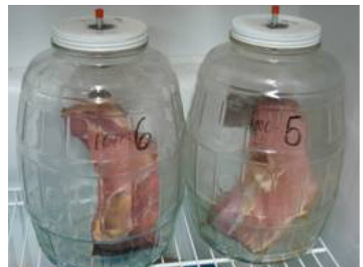
Left, laboratory dose-response bioassays assess mortality of known numbers and life stages of beetles and mites to different concentrations for phosphine gas for 48 hrs at 23 degrees C.
